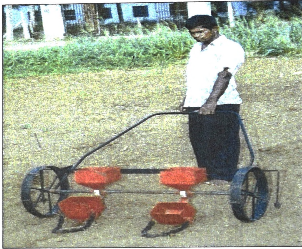
Manual Seeder for maize, green gram, black gram and soybean Photo Credit: FMRC
