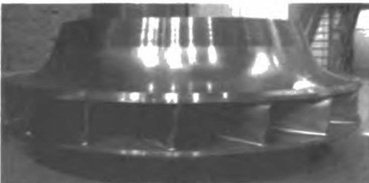
Fig 2-13 Prototype runner showing inlet
