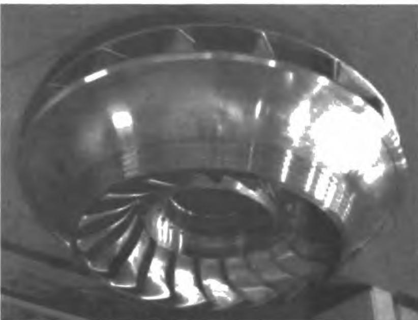
Fig 2-14 Proto type runner showing outlet
