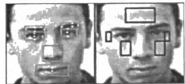
(a)Primary features (b) Secondary features Figure4: Features of interest
