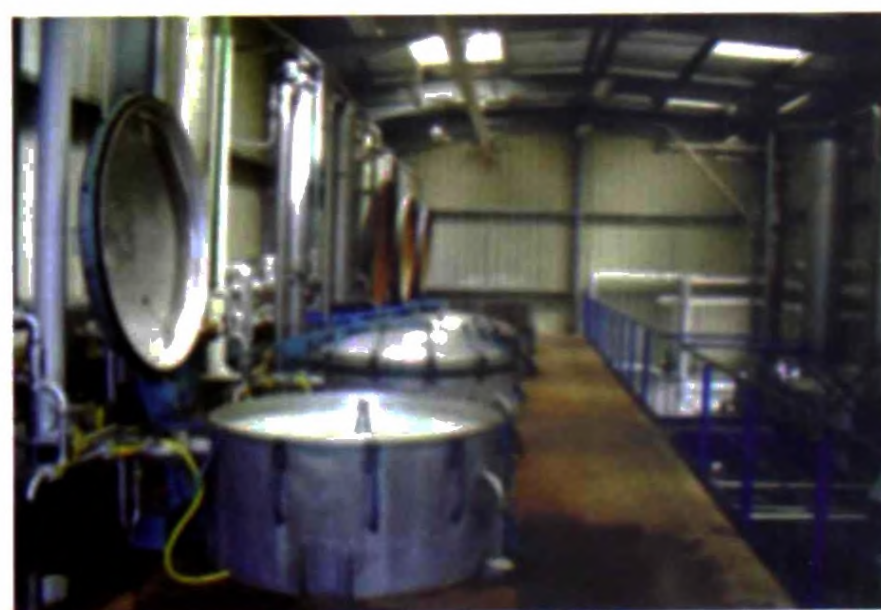
A modern commercial Lavender Distillation Assembly.
