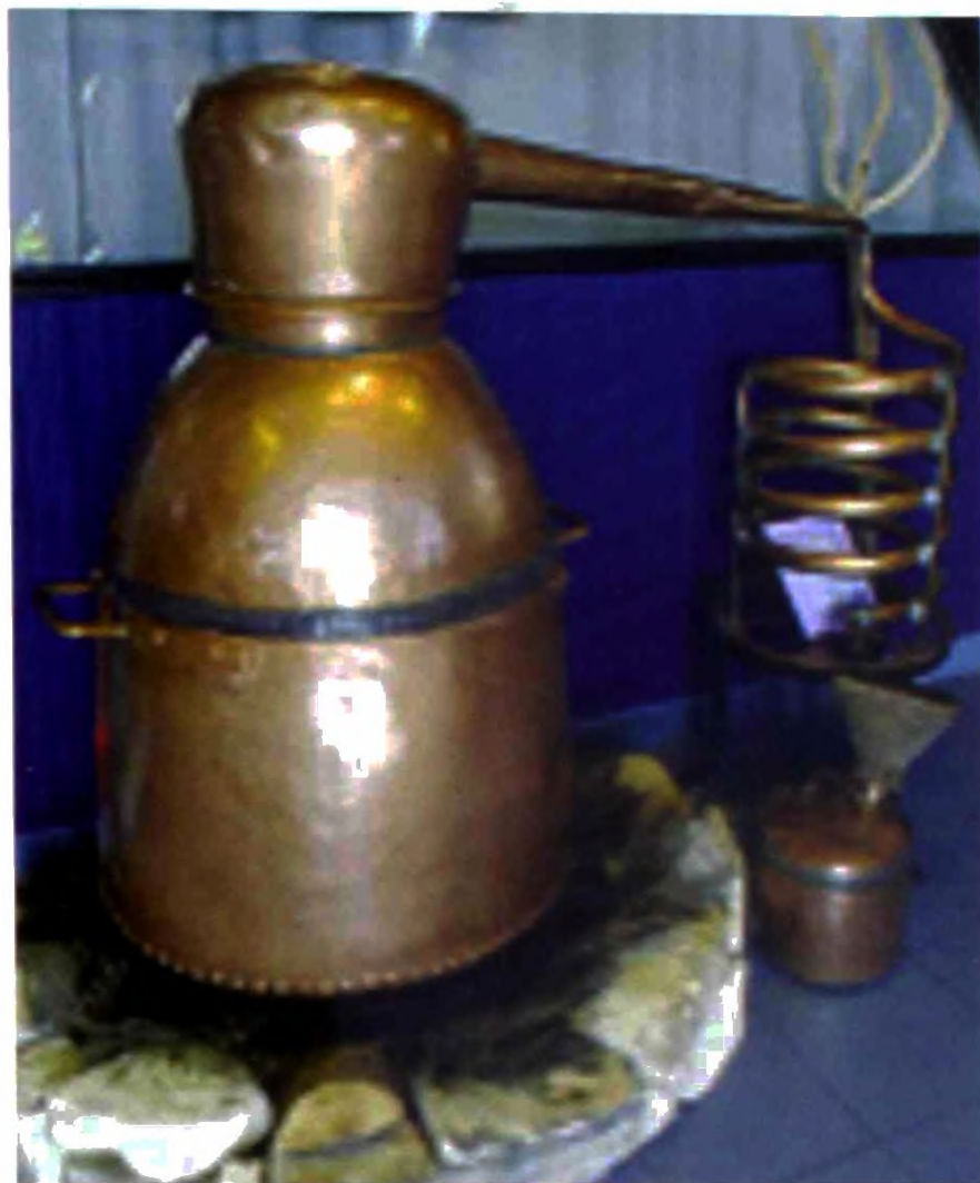
An Alembic : Home distillation unit
