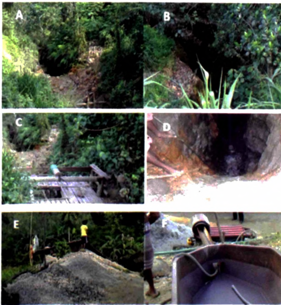
Fig. 7 Gem mining at Yakkalamulla site. (a) The minor valley where the host pegmatite is exposed; (b) A mined out area; (c) and (d) The mine shaft; (e) mine dumps consisting of pale colored pegmatitic materials; (f) A mechanical shaker used to separate stones
