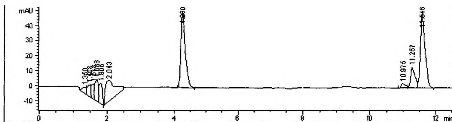
Figure A17. HPLC chromatogram of a solution of ferulic acid and curcumin (254 nm)
