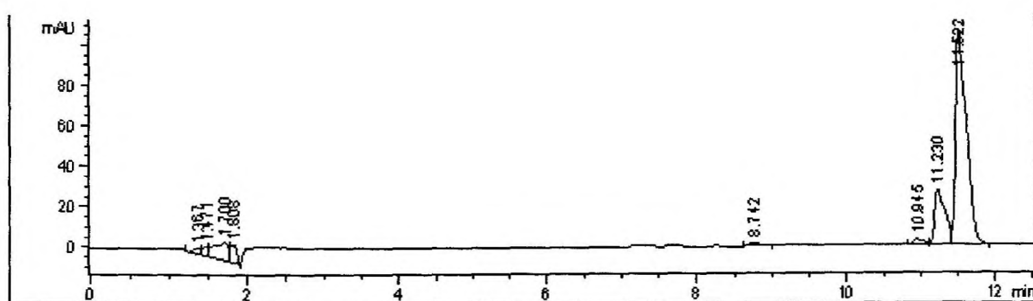
Figure A24. HPLC chromatogram of a solution of ferulic acid and curcumin after 8 h of UV irradiation (425 nm)
