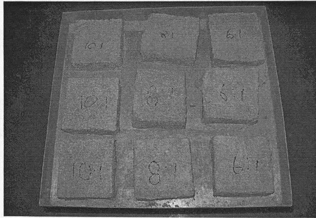
Figure78: Bricks produced by glass sand and cement
