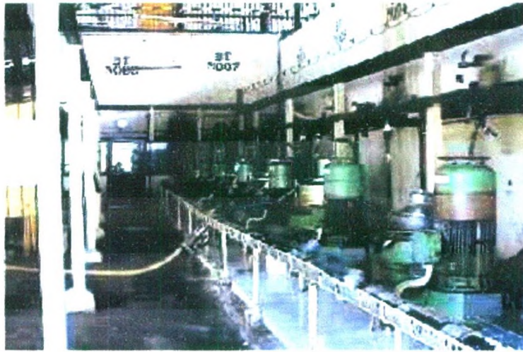
Centrifuges and square bulking tanks
