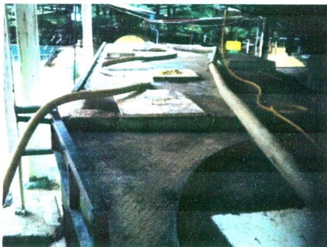
Long hoses used for latex transferring
