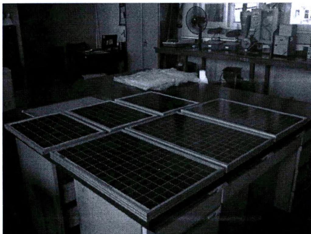
Figure 15. 20W and 30W photovoltaic cells bought
