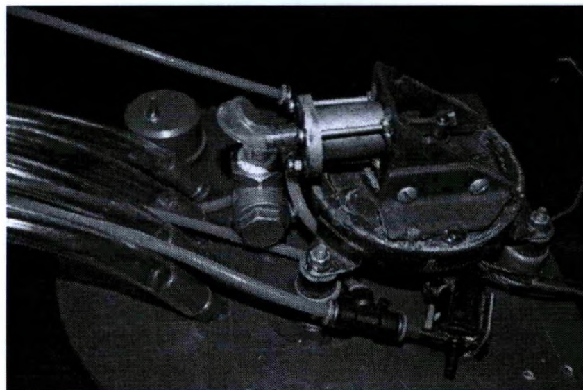
Figure 10. Arrangement of pulsation mechanism with PU pipes and fittings
