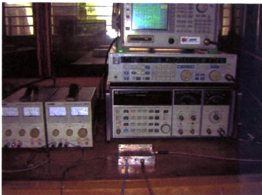
Figure 3.v.A10: Experimental set up for measuring the conversion gain.
