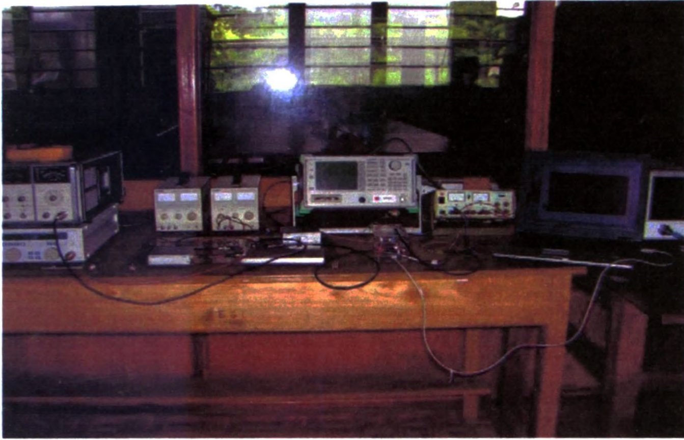
Fig. 7: Photograph of the Signal Meter with External Signal Generators and Power Supplies
