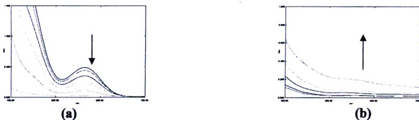
(a) UV-Visible spectra with the addition of 0.1M HCl (a) micro drop wise into a methanolic solution of the N,N- ethylenebis(acetylacetonimine)Ni(II) complex (b) UV-Visible spectra with the addition of 0.1 M NaOH micro drop wise into the same (acidified) solution of N,N- ethylenebis(acetylacetonimine)Ni(II) complex
