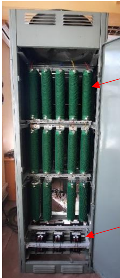
Internal view of the resistors and inductors used to develop the line model
