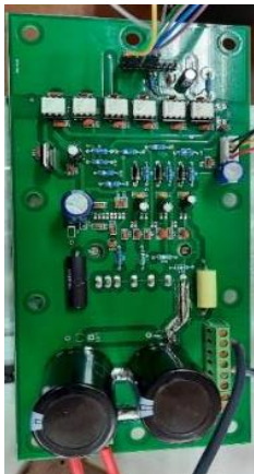
Fabricated circuit for re-phasing inverter
