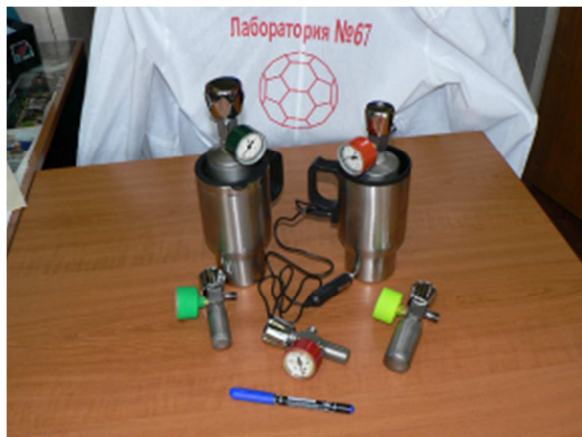
Fig. 7. "Dmisch" hydrogen storage devices equipped with heat exchangers powered by 12V DC sources.
