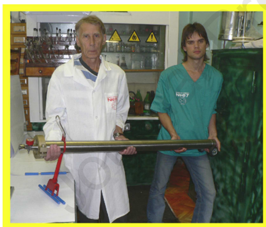
Fig. 8. Laboratory storage of high pressure hydrogen with a capacity of 2000 liters of hydrogen.
