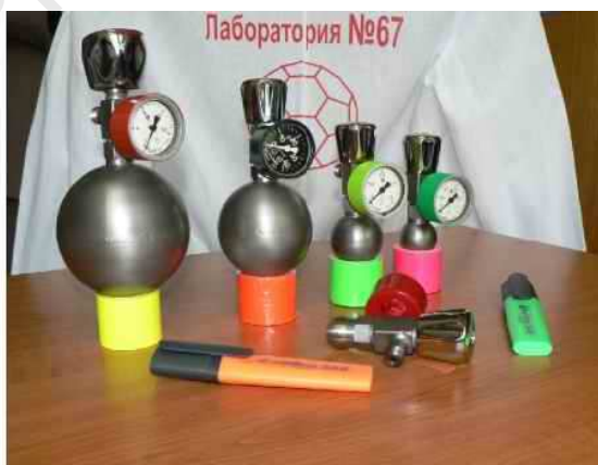
Fig. 4. "Alsav" hydrogen storage tanks with a hydrogen capacity of 3, 10, 15, 75 and 175 liters.
