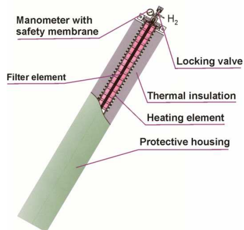
Fig. 8. Laboratory storage of high pressure hydrogen with a capacity of 2000 liters of hydrogen.
