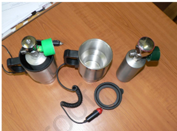
Fig. 7. "Dmisch" hydrogen storage devices equipped with heat exchangers powered by 12V DC sources.
