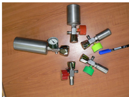
Fig. 4. "Alsav" hydrogen storage tanks with a hydrogen capacity of 3, 10, 15, 75 and 175 liters.
