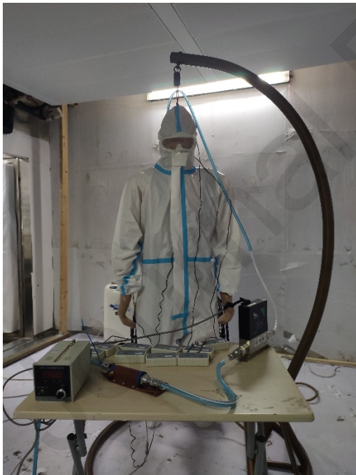
Fig. 2. MUPC air supply performance experimental setup
